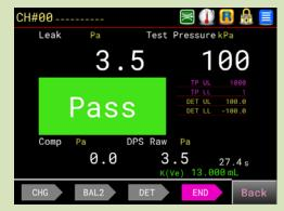
Measurement screen is selectable from 6 different screens. For four measurement screens, "Standard", "Simple", "Waveform" and "4-Channel", the items to be displayed can be customized.
