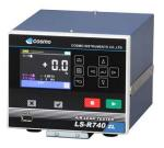
LS-R740ZL tests the airtightness of sealed products. The part to be tested is placed in a capsule and pressurized to measure the pressure change caused by leak flowing into the part.
